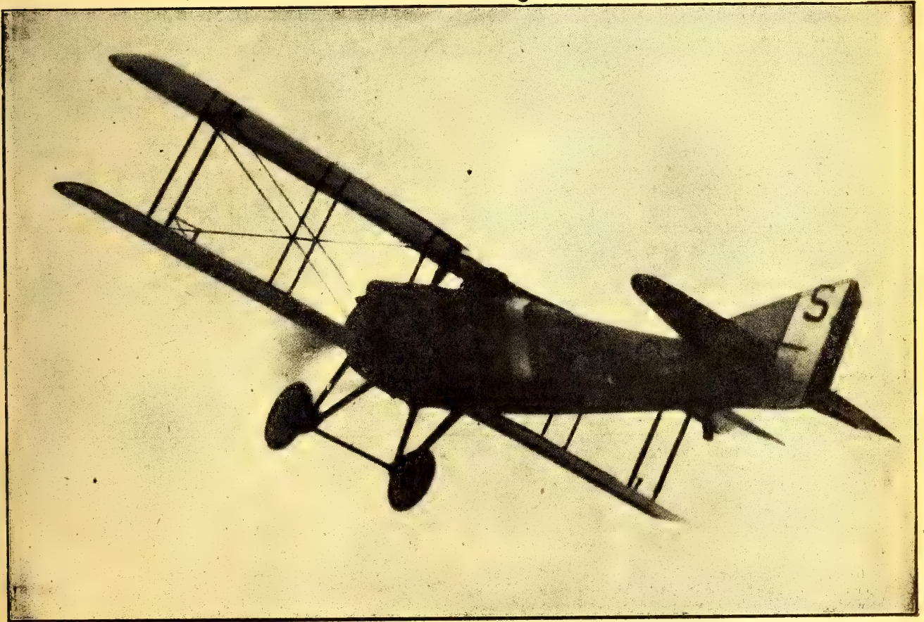
THE S.P.A.D. SINGLE-SEATER.—A standard French fighting machine, which is also used considerably by other Allies.
